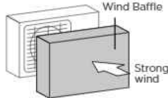
Build a wind Baffle to protect the unit
