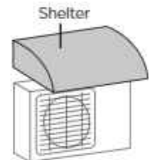
Build a shelter to protect the unit
