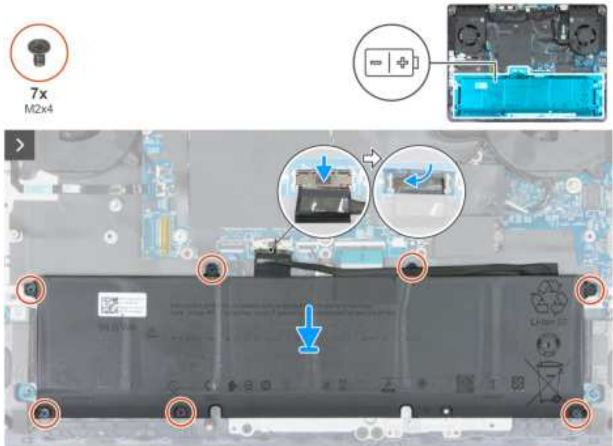
Figure 20. Installing the battery
