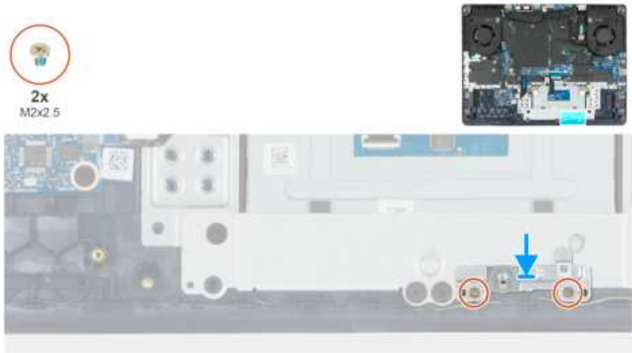
Figure 44. Installing the battery bracket
