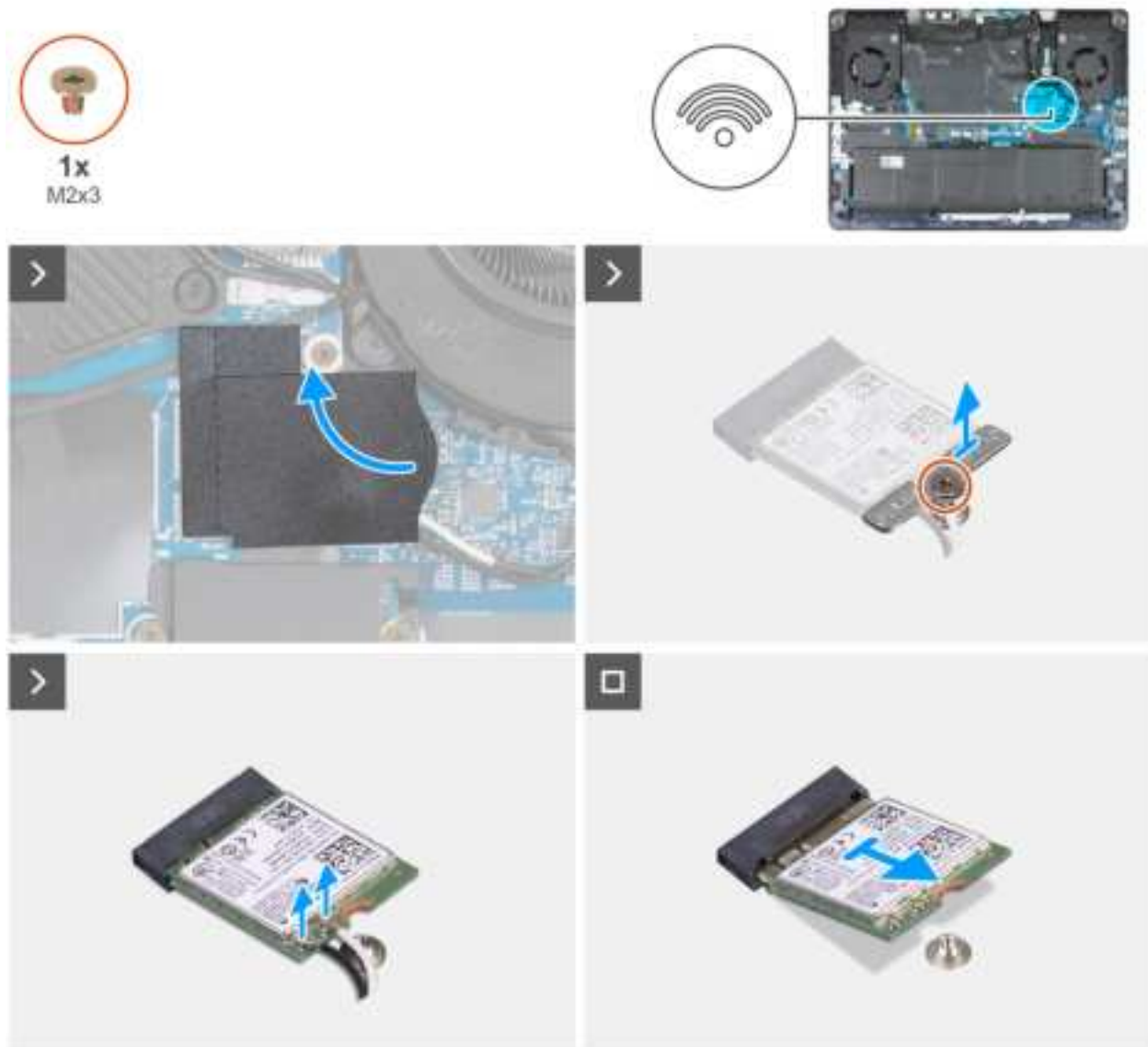
Figure 35. Removing the wireless card
