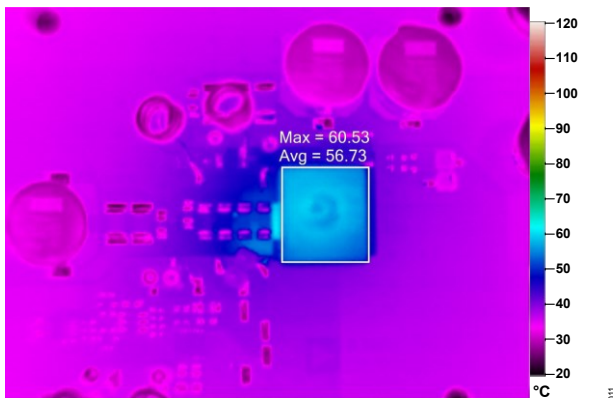
Figure 11. Thermal Image of Bottom Layer at V_{OUT} = 24V , I_{OUT} = 6A , F_{sw} = 1MHz (Thermal Values are on L1)
