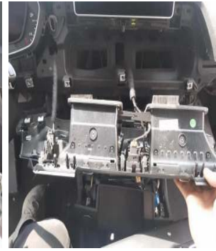
取下风口装饰板并拔下风口插头/Remove the air vent decorative panel and unplug the air vent plug
