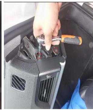
用套筒取下两颗螺丝 /Remove two screws with a socket
