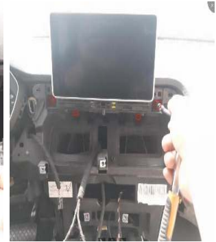
取下显示屏固定螺丝/Remove the fixing screws of the display screen
