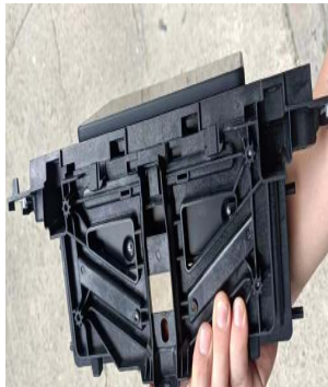
取下风口装饰板并拔下风口插头/Remove the air vent decorative panel and unplug the air vent plug
