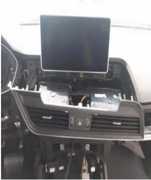
取下风口装饰板并拔下风口插头/Remove the air vent decorative panel and unplug the air vent plug
