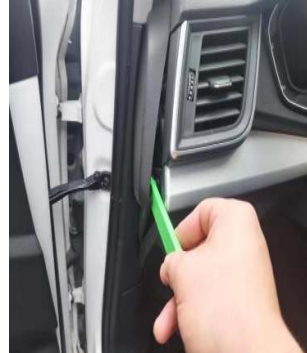
用撬板取下主驾驶左侧板/Remove the driver's left side panel with a pry bar
