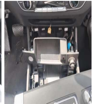
取下小储物盒并取下插 头/Remove the small storage box and remove the plug
