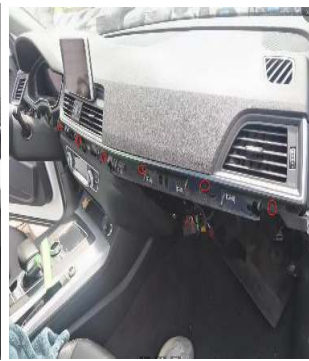
用套筒取下红色标记的螺丝/Remove the screw marked in red with a socket
