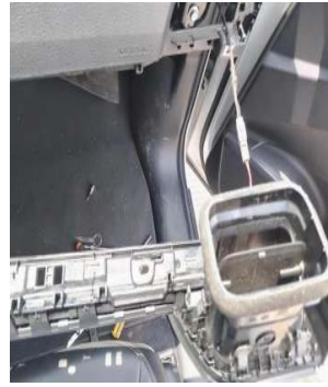
取下风口装饰板并拔下风口插头/Remove the air vent decorative panel and unplug the air vent plug
