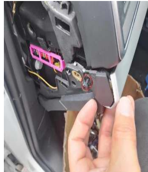
用螺丝刀取下装饰条固定螺丝/Use a screwdriver to remove the decorative strip fixing screw
