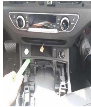
移开档把装饰板再撬下 小储物盒/Move the gear aside, remove the decorative panel, and pry off the small storage box
