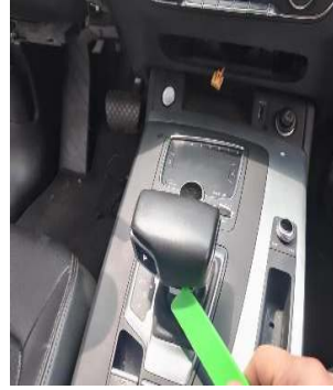
撬开档把盖/Pry open the gear lever cover
