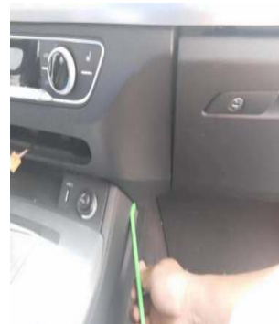
撬下空调控制面板/Pry off the air conditioning control pan
