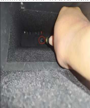
取下主驾驶小储物盒固定螺丝/Remove the fixing screws of the driver's small storage box
