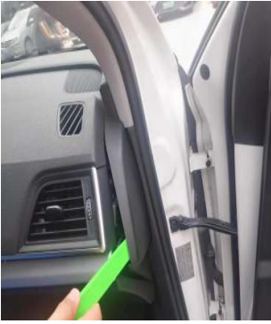
用撬板把右侧板拆下 /Remove the right side panel with a pry bar
