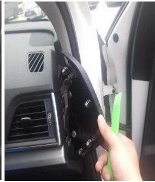
取下右侧板/Remove the right side panel
