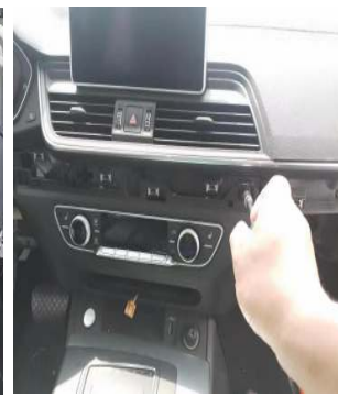
取下螺丝/Remove the screw
