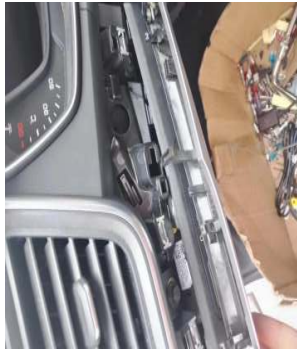
撬松装饰条后向左移动一下再取下装饰条/Loosen the decorative strip and
