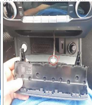
取下主驾驶装饰护板固定螺丝/Remove the fixing screws of the driver's decorative
