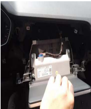
取下风口装饰板并拔下风口插头/Remove the air vent decorative panel and unplug the air vent plug
