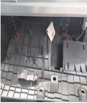
取下储物盒并把储物盒电源插头取下/Remove the storage box and disconnect the power plug from the storage box
