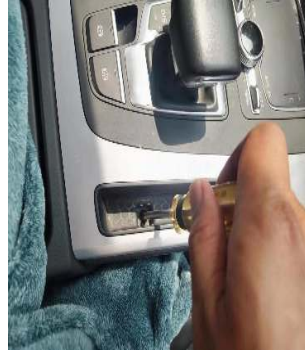
撬开档把小垫片并取下 螺丝/Pry open the gear lever and remove the small gasket and screw
