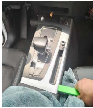
撬开档把小垫片并取下 螺丝/Pry open the gear lever and remove the small gasket and screw
