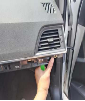
撬下风口装饰板/Pry off the air vent decorative panel
