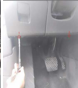
取下主驾驶装饰护板固定螺丝/Remove the fixing screws of the driver's decorative
