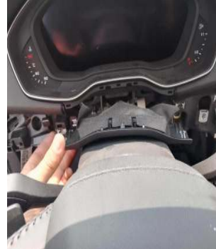
用螺丝刀取下装饰条固定螺丝/Use a screwdriver to remove the decorative strip fixing screw
