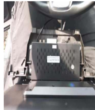
取下风口装饰板并拔下风口插头/Remove the air vent decorative panel and unplug the air vent plug
