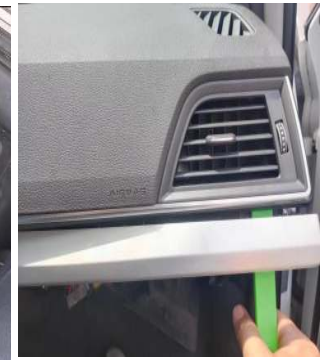
用撬板取下银色装饰条 /Use a pry to remove the silver decorative strip
