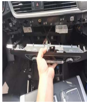
移开档把装饰板再撬下 小储物盒/Move the gear aside, remove the decorative panel, and pry off the small storage box
