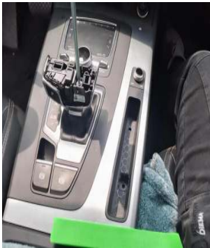
再取下按键后面螺丝 /Remove the screw behind the button again
