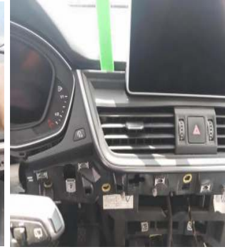
撬下风口装饰板/Pry off the air vent decorative panel
