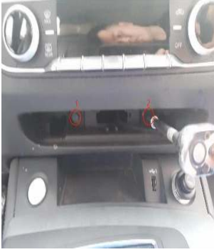
再取下按键后面螺丝 /Remove the screw behind the button again
