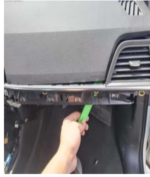
撬下风口装饰板/Pry off the air vent decorative panel
