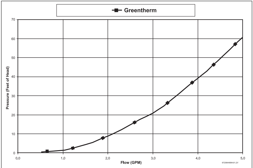
Fig. 45 Pressure drop curve
