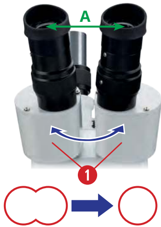
Fig. 6: Adjust the interpupillary distance.
