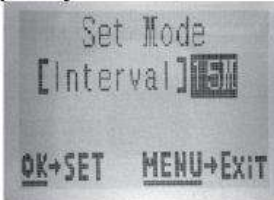
Schritt 7: Field-Scan-Intervall einstellen [Step 7]-set Field Scan Interval
