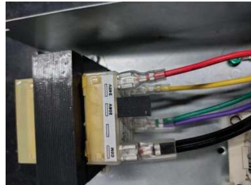
Fig. 6 – Red Wire to 240V, Black Wire to COM
