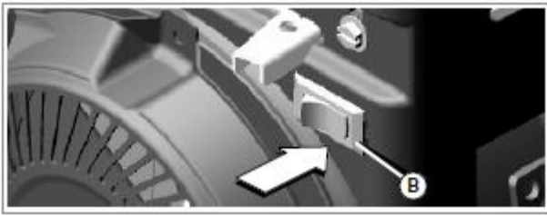
Fig. 24 – Select the 'ON' position on the engine switch control
