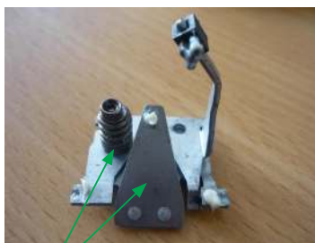
Danfoss Main arm with torx screw Spring steel
