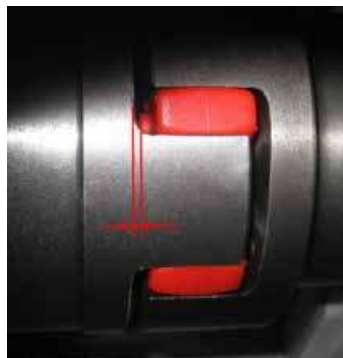
1. Coupling distance (check before disassembling)
