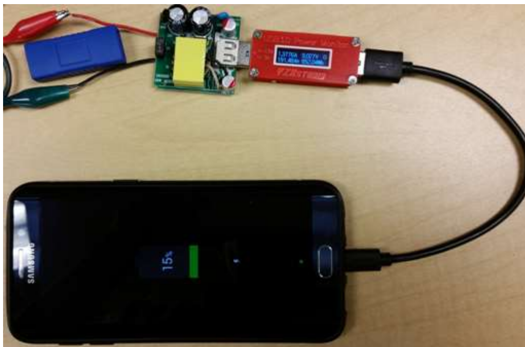
Figure 9: the connection between the 18W QC3.0 Evaluation Board to a QC3.0-equipped smart phone
