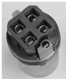
Style 1 ground conductor attaches to shell
