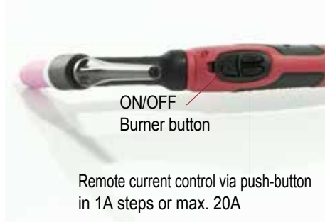
TIG hosepack with UP/DOWN pushbutton / switch module (3DT) (= standard)
