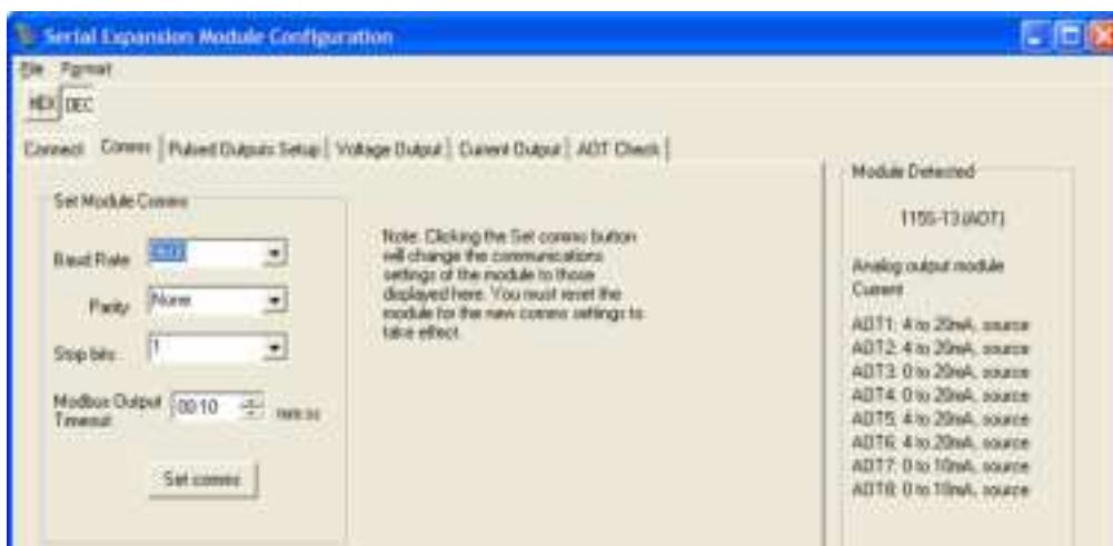
Figure 4-2: Communications configuration screen.
