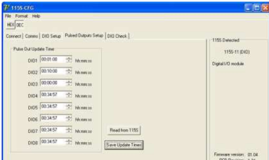
Figure 4-3: Pulsed outputs setup page for a 115S-11. The pulsed outputs are available on all models.
