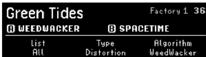
Fig. 6.1 The upper right corner displays the List and location of the Program.
