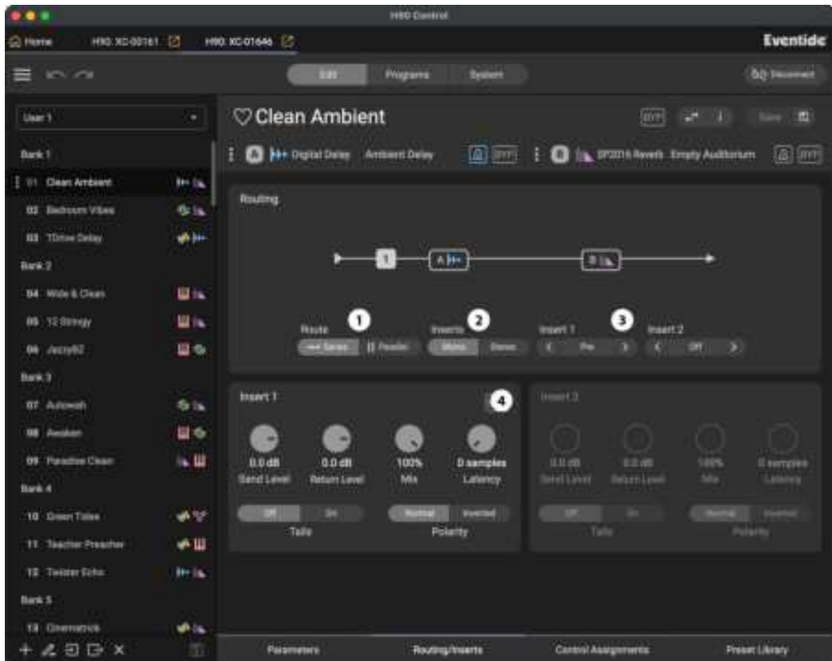
Fig. 10.8 The Routing/Inserts edit menu. Insert 1 is Pre Preset A.
