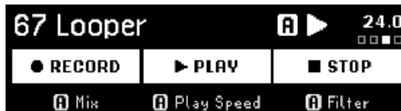
Fig. 3 The Looper displays A in the top right corner when loaded into Preset slot A.
