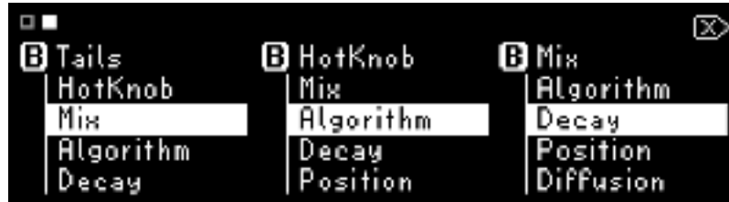
Fig. 5.9 Page 2 of the Quick Knob assignment menu; press any Quick Knob to toggle pages.
