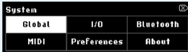
Fig. 7.11 Press and hold the Programs and Routing buttons to enter the H90's System Menu.
