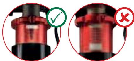
Maximum preload setting for brake pedal Left: Correct, right: wrong!
