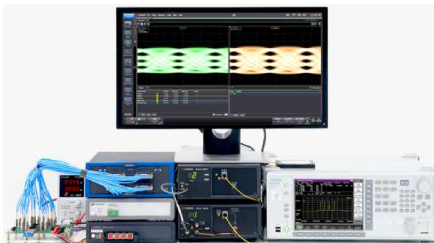
The above shows the optical eye diagram output results of the PAM4 optical module from the FS laboratory.
