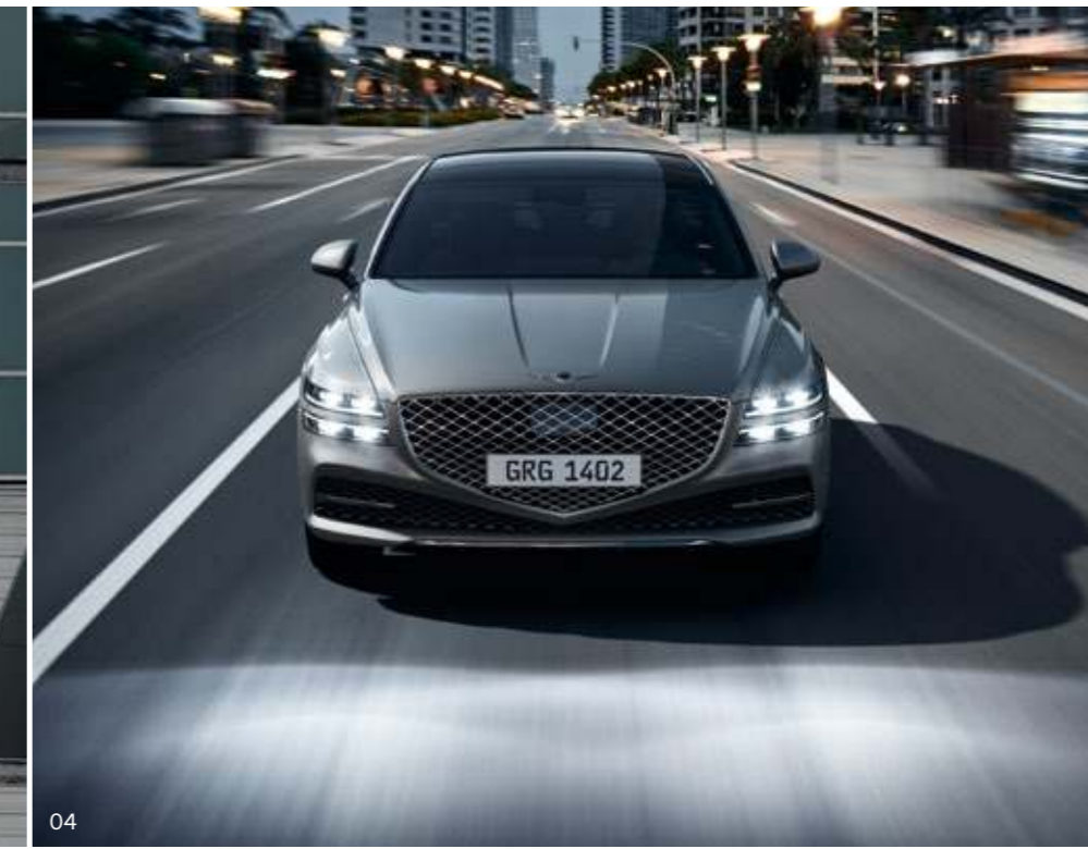
04. Intelligent Front-Lighting System (IFS) _ This system automatically activates or deactivates part of the high beam lights when it detects an oncoming vehicle or a vehicle ahead, to prevent glare for drivers of other vehicles. This supports safer driving at night as the high beam lights don't have to be adjusted manually.
