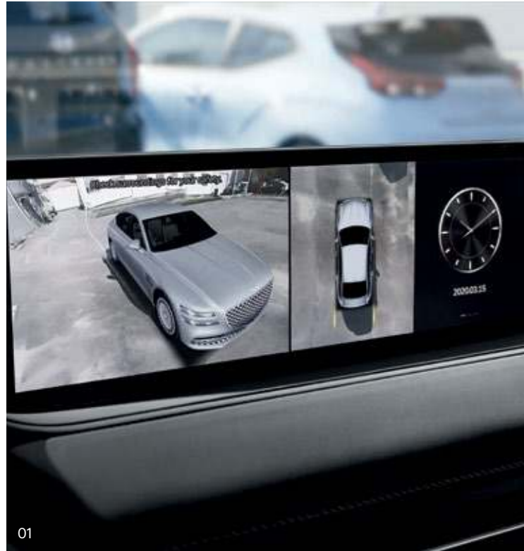
01. Surround View Monitor (SVM) system _ Video images of the area surrounding the vehicle can be viewed to assist in safe parking.
