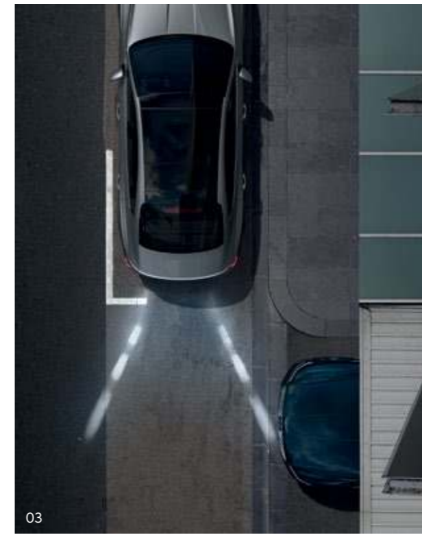
03. Reverse guiding lamps _ When in reverse, these LED lights are angled to illuminate the ground behind the vehicle. This allows pedestrians and other vehicles to easily notice that the vehicle is reversing, maximizing safety and preventing accidents.
