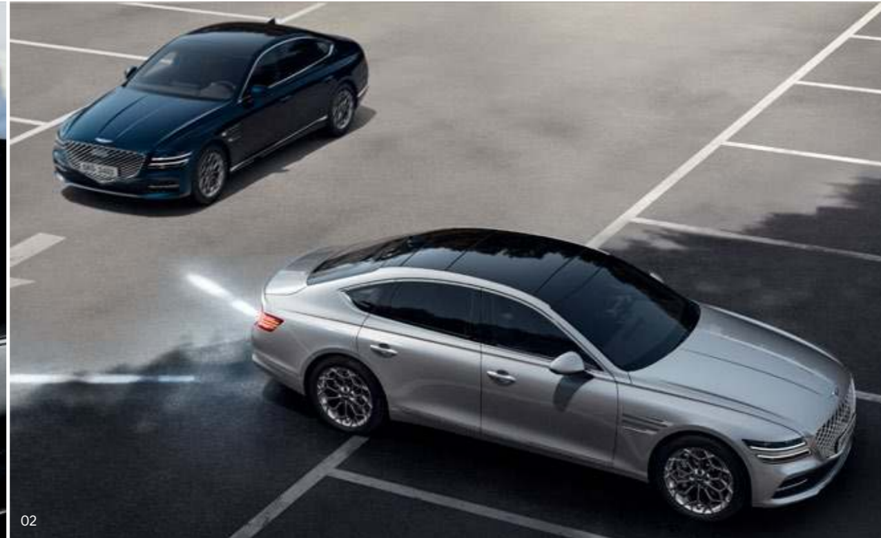
02. Rear Cross-Traffic Collision-Avoidance Assist (RCCA) system _ This system alerts the driver if a collision risk is detected from the left and right sides of the vehicle while reversing. If the risk increases even after the warning, RCCA helps to stop the vehicle.
