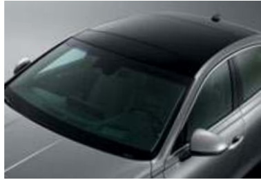
Double-jointed soundproof glass (windshield and all doors)
