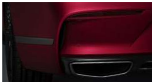
Rear bumper side air vent & edge
