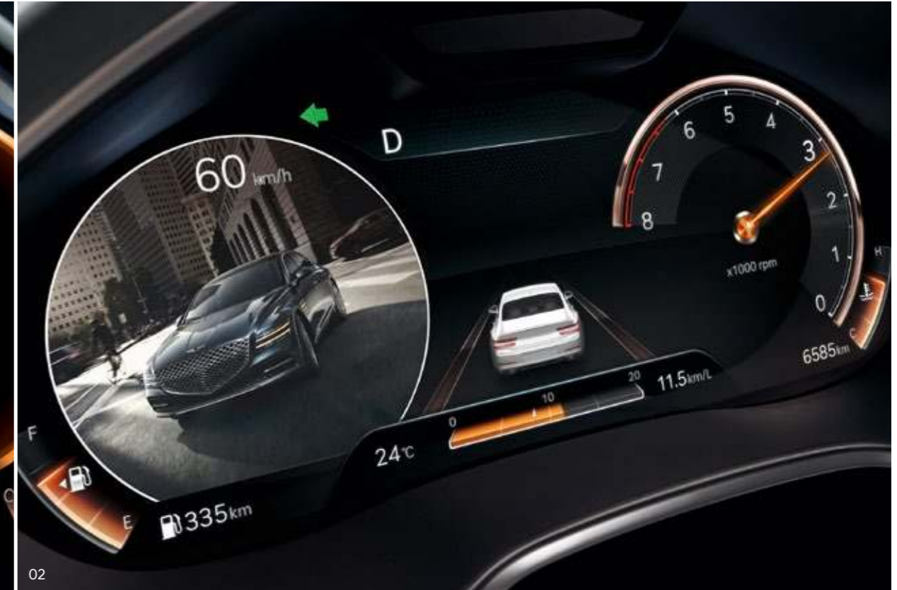
02. Blind-Spot View Monitor (BVM) system _ When the turn signals are activated, video images of the respective side/rear view of the vehicle appears on the center cluster.
