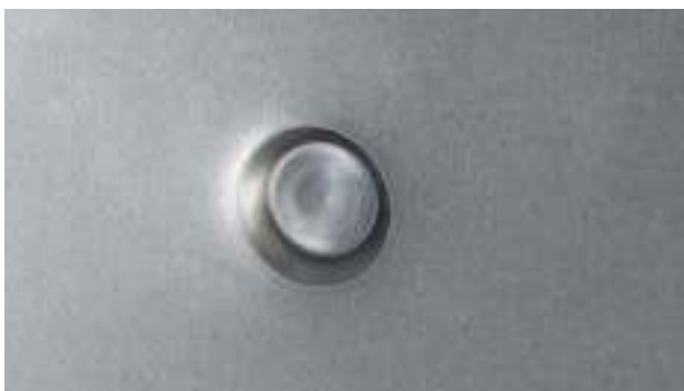
RESULT OF THE INSTALLATION OF SELF-PIERCING RIVET
