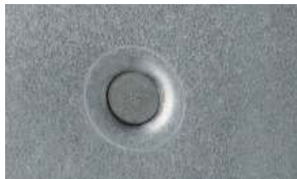
RESULT OF THE INSTALLATION OF SELF-PIERCING RIVET
