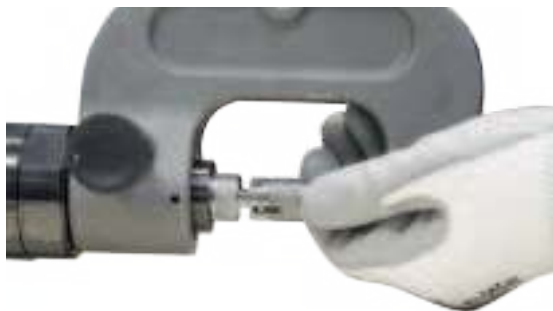
Using the screw, fasten the extension supplied with the arm.
