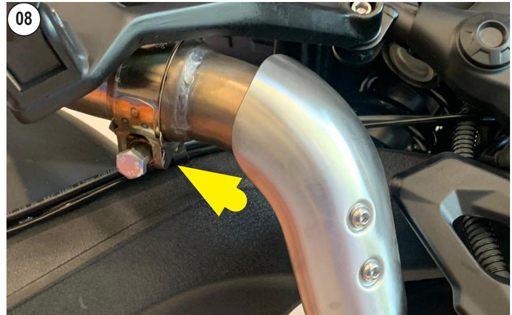
SCREW THE STOCK CLAMP
