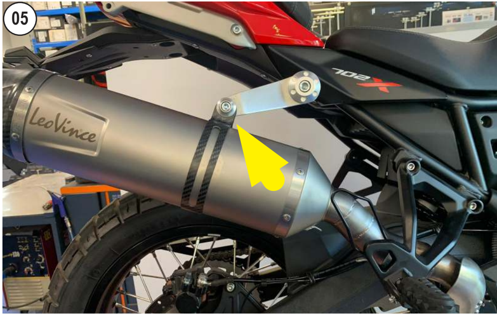
FIT THE LeoVince MUFFLER AND SCREW
