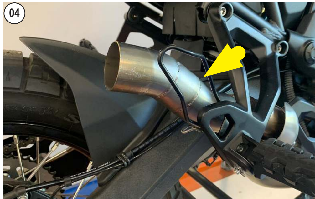
INSTALL THE LeoVince PIPE
