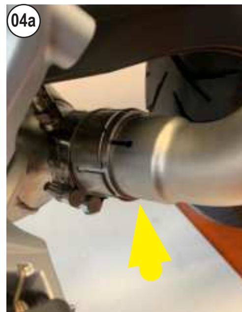
INSTALL THE LEOVINCE PIPE ON THE STOCK PIPE
