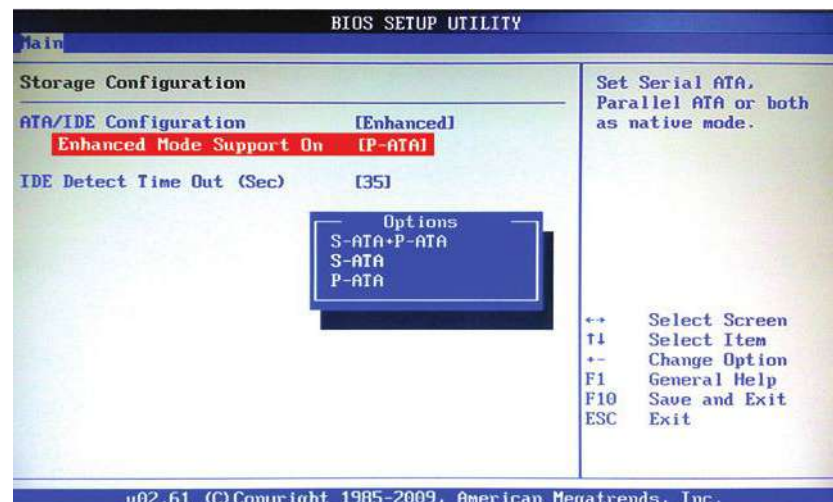
[Figure 3-4] Storage Configuration
