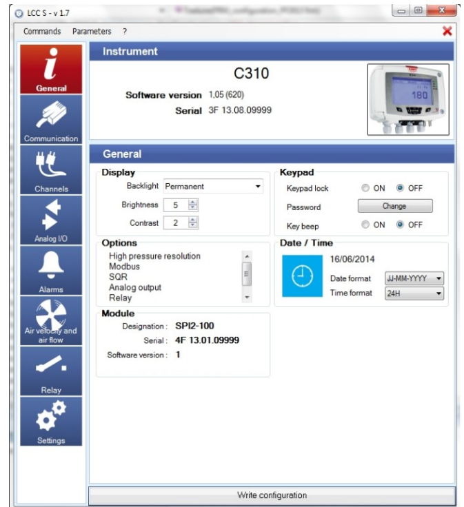
"General" panel for a class 310 transmitter
