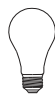
Light Bulb (A19 100 watt maximum) Ampoule (A19 100 watts maximum) Bombilla (A19 100 vatios máximo)
