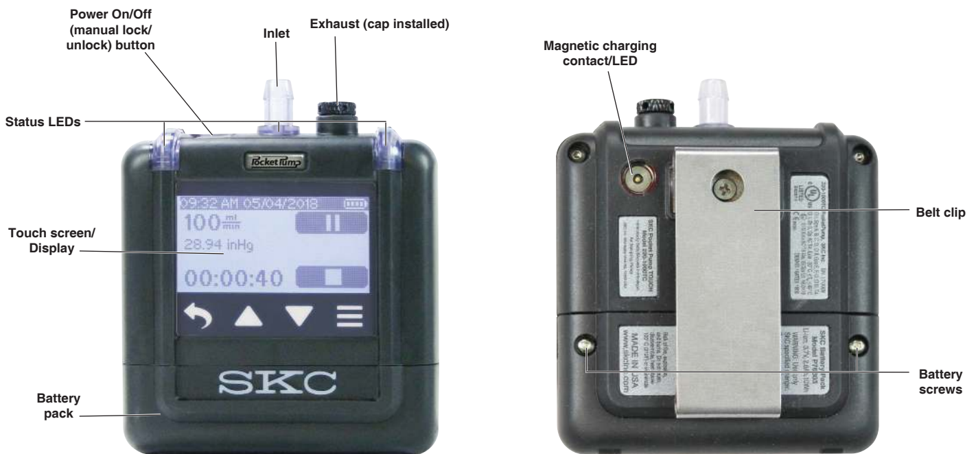
Figure 1. Pocket Pump TOUCH Physical Feature Overview
