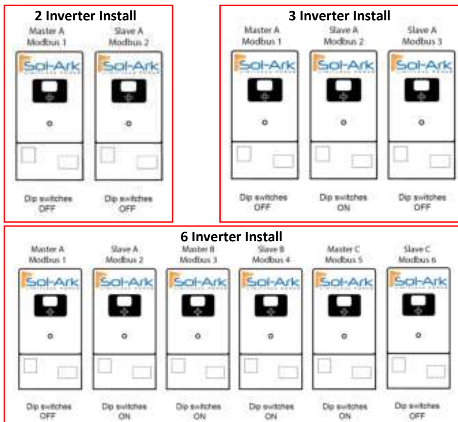
Fig. F – Dipswitch positions (OFF = Down | ON = Up)
