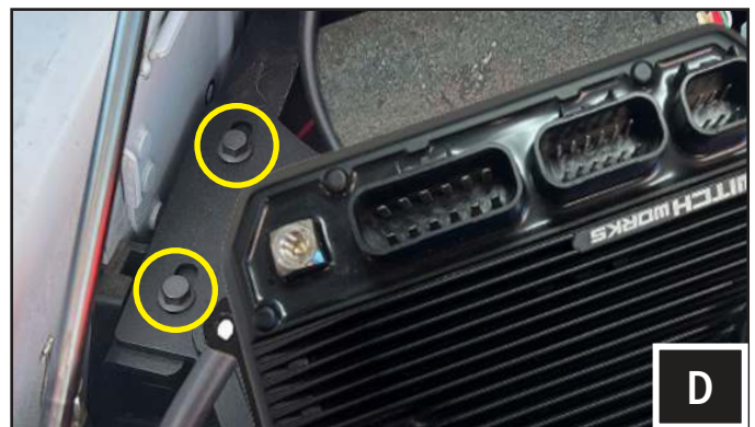
D. Attach the module bracket to the fender bracket using the supplied M6-1x12mm hex head bolts (B-S2870).
