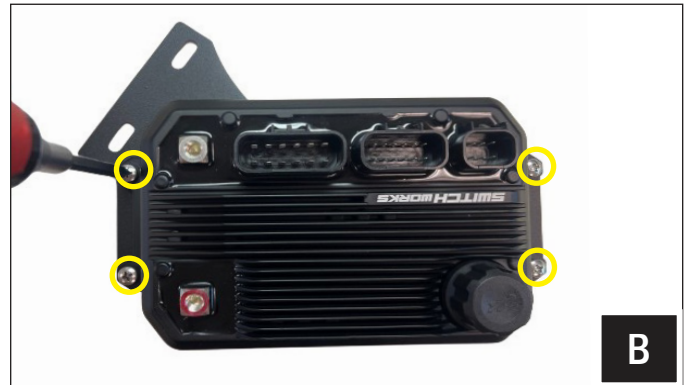
B. Mount the SWITCH Works brain module to the B-MB3192 bracket using the supplied M5x10mm screw (x4).
