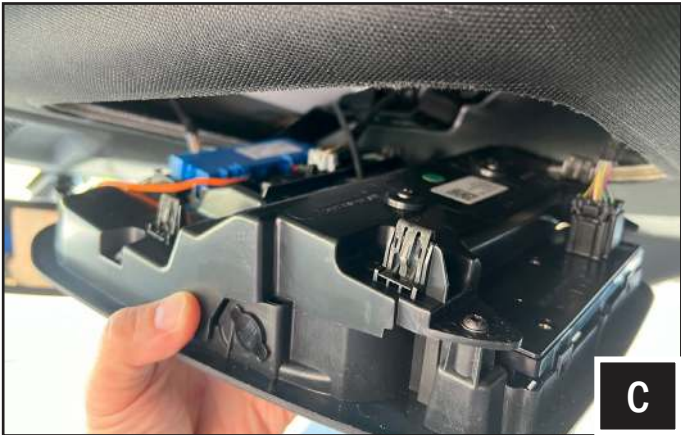
C. Pull down the overhead console and unplug the connectors.
