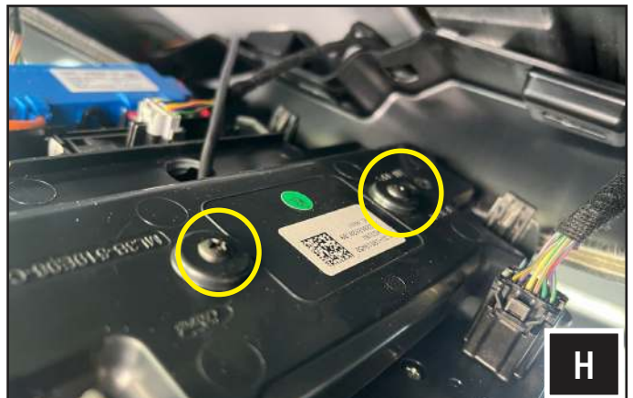
H. Secure the F150 Raptor Fascia to the sunglass holder cavity using the #7-19x.75 Phillips screws and M4 flat washers (x2 each).
