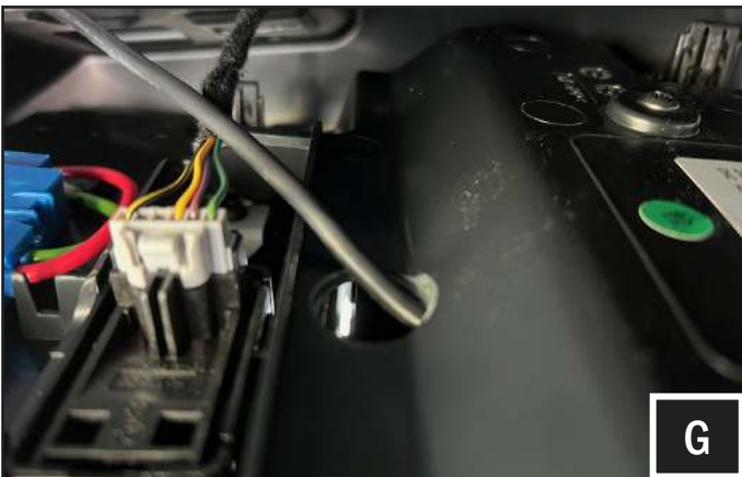
G. Route the controller cable through the hole drilled on the overhead console and run it towards the passenger side A pillar.
