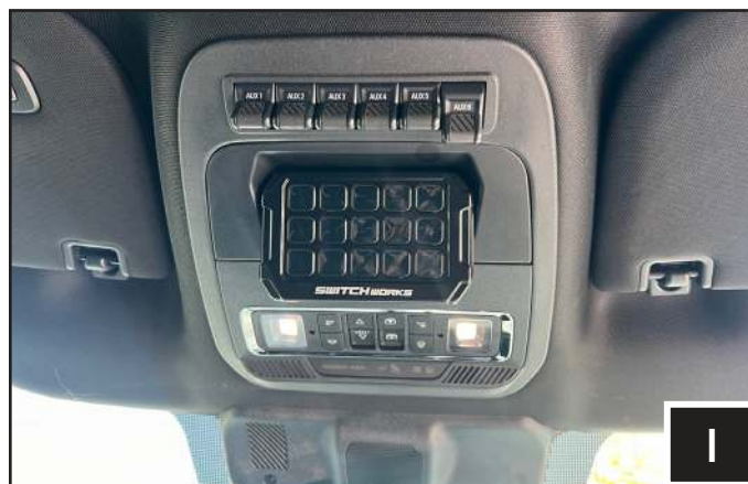
I. Plug the connectors and re-install the overhead console.
