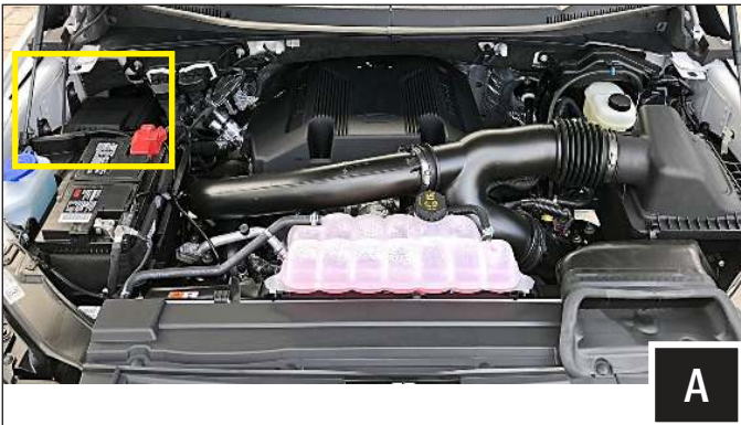
A. The SWITCH Works brain module is mounted in this area of the engine bay above the fusebox.
