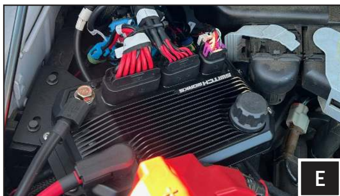
E. Connect the accessories to be used to the High and Low current harnesses and plug the harnesses to the brain module. NOTE that the 15 button controller MUST be plugged in to the module before connecting the power and ground cables to the battery. Snap on the terminal cover to the module's + terminal.
