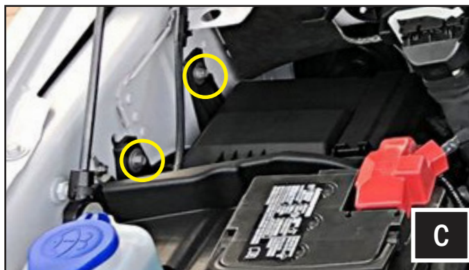
C. Mount the fender bracket (B-MB3191) to the fender wall (above the fusebox) using the factory bolts.
