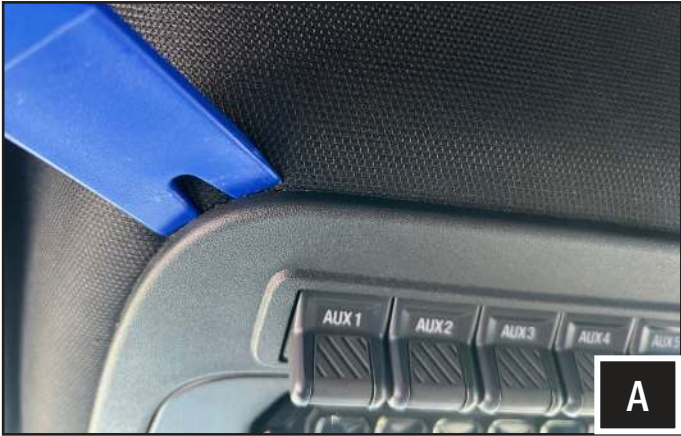
A. Remove the overhead console by using a plastic pry tool carefully working all around the console.
