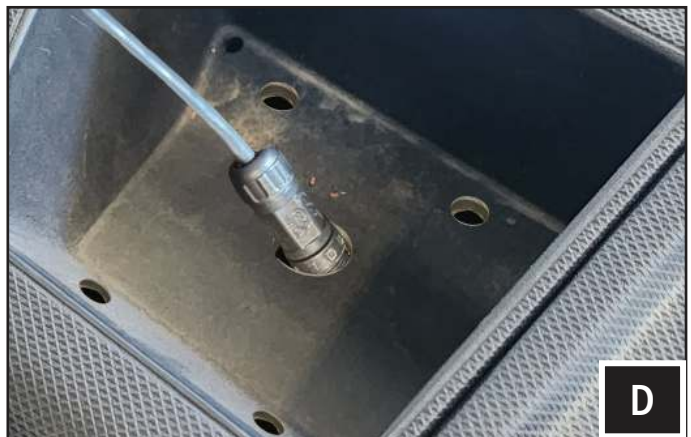
D. Insert the 15-button controller cable through the middle hole in the dash pocket.
