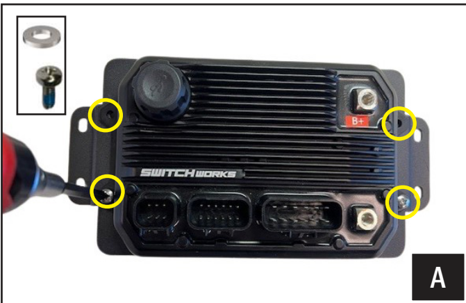
A. Mount the ALPHA12 Brain module to the Ranger brain module bracket [B-A3293] using (4) M5x10mm Phillips screws [B-S1158] and washers.
