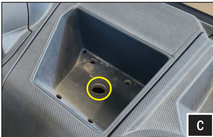
C. Drill a 5/8" hole in the middle of the dash pocket for the controller cable.
