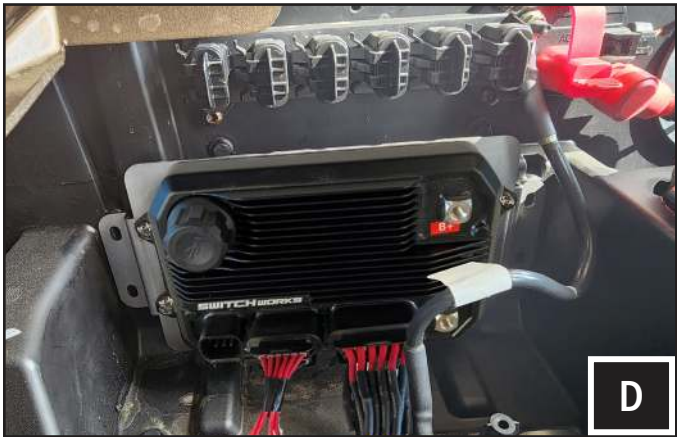
H. Connect the accessories to the High and Low current harnesses and plug the harnesses to the brain module. NOTE that the 15 button controller MUST be plugged in to the module before connecting the power and ground cables to the battery. Snap on the terminal cover to the module's + terminal.
