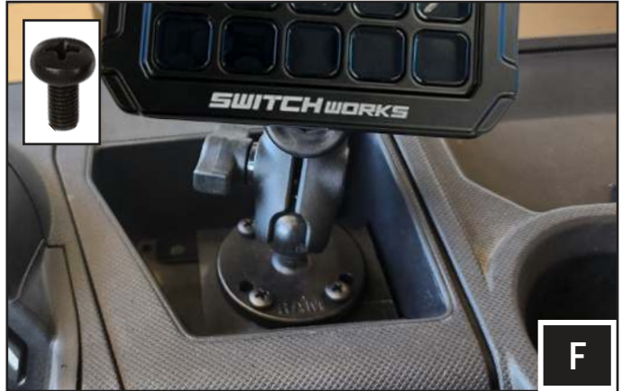
F. Mount the 15-button with RAM Mount to the mounting plate using (4) M5x16mm Pan-Head screws (B-S2708) included in the ALPHA12 kit.
