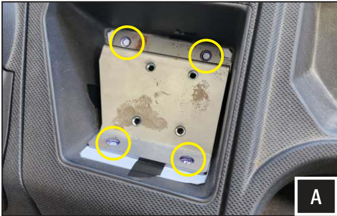
A. Place the Ranger RAM Mount mounting plate in the dash pocket and mark drill holes on the 4 corner holes .
