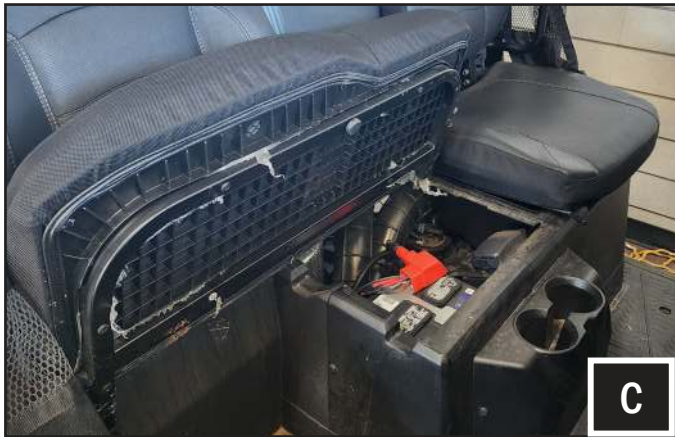
C. Run the power and ground wires from the ALPHA12 kit to the battery location. Battery is located under the front passenger seat on 2-door models and under the rear passenger seat in 4 door models.
