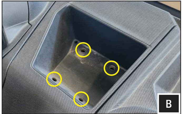
B. Drill (4) holes for the push rivets using a 5/16"holes drill bit.
