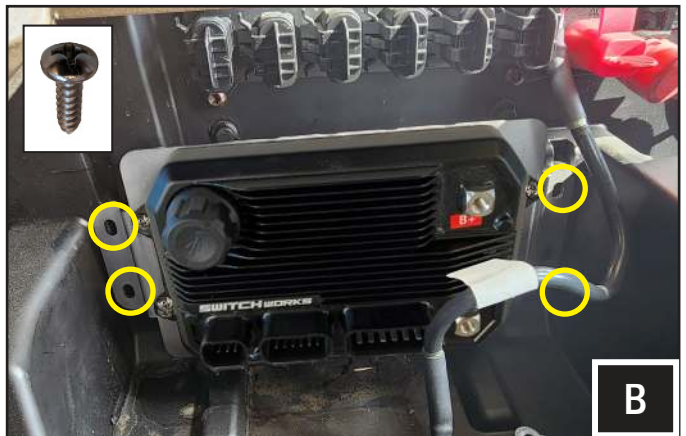
B. Use the (4) #12x0.75" self tapping Phillips screws [B-HP3300], included in the kit, to secure the Ranger brain bracket to firewall below the busbar. Line up the bracket holes to the pre-existing screw bosses.
