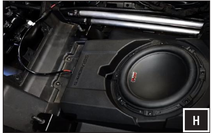
H. Make sure the subwoofer cable is tucked away from the seat bolts.
