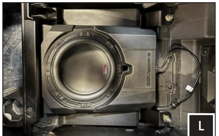
L. Installation shown is manual was done under the driver seat, installation under the passenger seat will have the same procedure.
