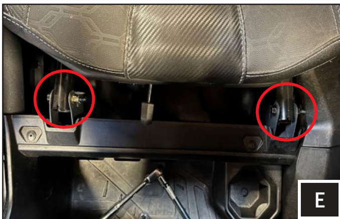
E. Remove the (2) 13mm bolt and nut on the front seat rail.
