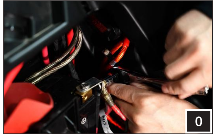
O. Connect the power wire to the battery positive and negative posts.
