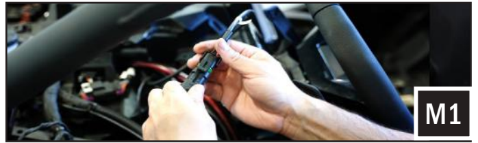
M. Plug in the amplifier's front speaker output to the B-H1385 "Y" harness and the rear speaker outputs to the B-H1913, 4-pin audio extension harness.
