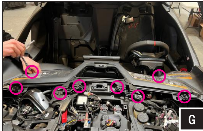
G. Remove the central dashboard.
