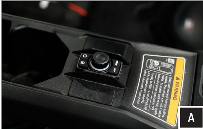
A. Install the LIT-CC RGB LED Controller Rocker Switch in an unoccupied rocker switch opening.
