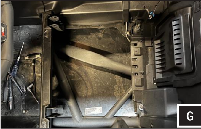
G. Carefully remove the seat.
