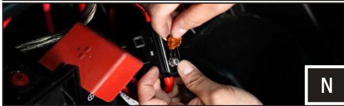
N. Install the fuse holder on the power wire no more than 18" away from the battery and install the fuse.
