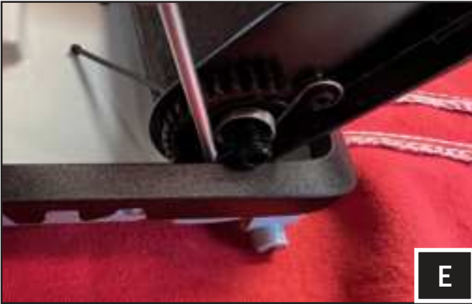
E. Use a small screw driver to carefully pry out the sunglasses holder from the overhead console.
