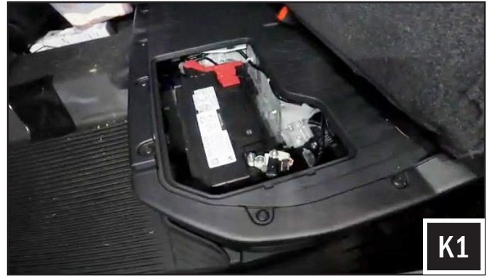
K. NOTE that the 15 button controller MUST be plugged in to the module before connecting the power cable to the battery. Run the power wire from the ALPHA12 brain module along the firewall towards the battery located under the driver side backseat [K1].
