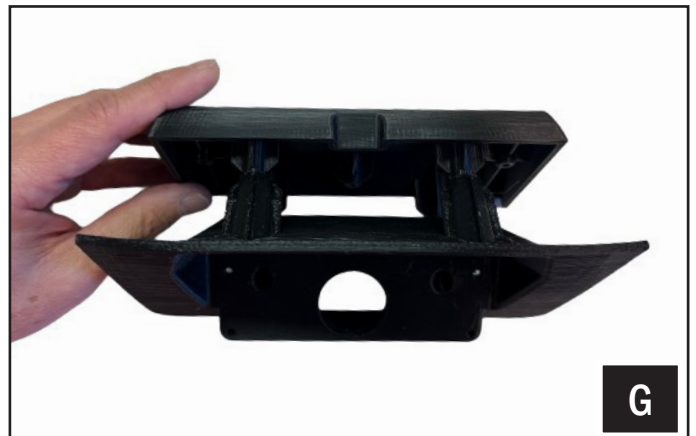
G. Assemble the Tundra fascia to the mounting bracket using the supplied (4) #7-19x3/4" Phillips screws (B-S1656).
