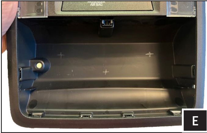
E. Mark the drill guides and drill 3 holes using a 3mm drill bit.
