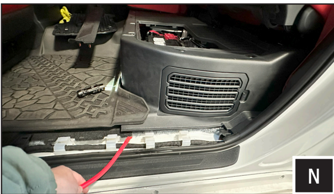
N. Insert the cable under the backseat bottom panel.
