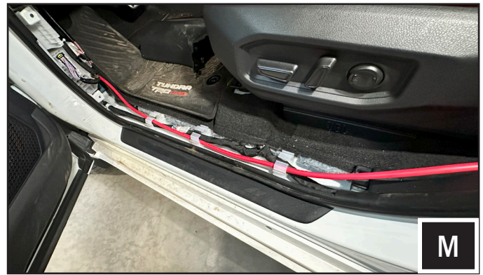
M. Run the power cable along the doorsill towards the backseat.
