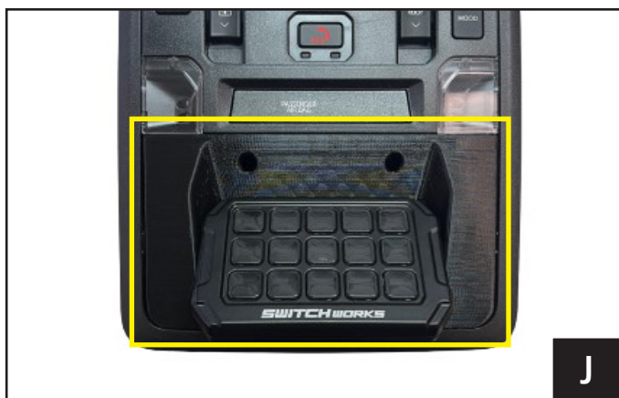
J. Insert the cable through the hole drilled on the overhead console and place the controller and bracket in the sunglasses holder cavity.
