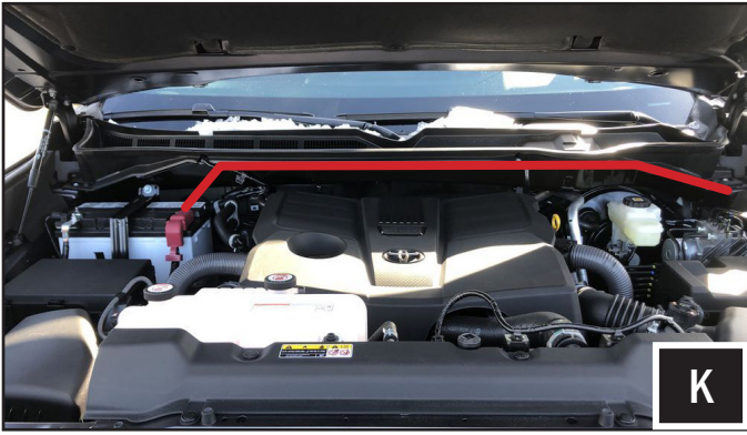
K. NOTE that the 15 button controller MUST be plugged in to the module before connecting the power cable to the battery. Run the power wire from the ALPHA12 brain module along the firewall towards the battery located under the driver side backseat [K1].
