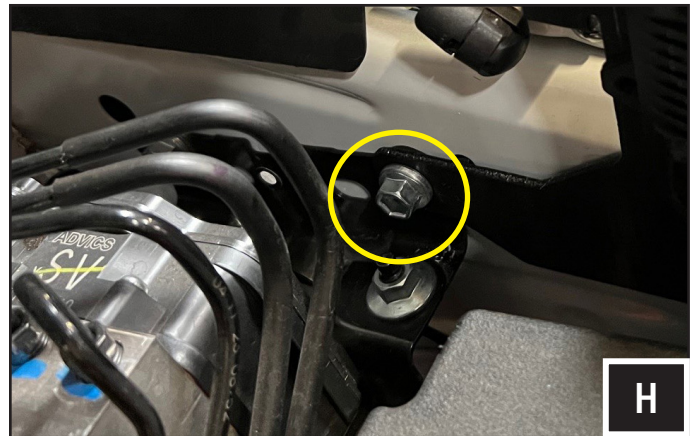
H. Position the bottom left tab of the ALPHA12 bracket to the ABS pump bracket and fasten using the factory bolt. Tighten all 3 mounting bolts to secure the ALPHA12 brain module.
