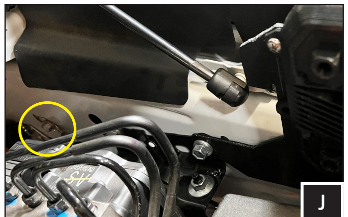
J. Connect the ground wire from the ALPHA12 brain module to the factory grounding point on the driver side fender.
