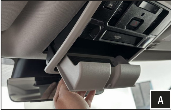
A. Use both hands and grab the back edge (edge closest to the windshield) of the overhead console. Pull down firmly until the back side snaps loose. Slide the console forward towards the windshield.
