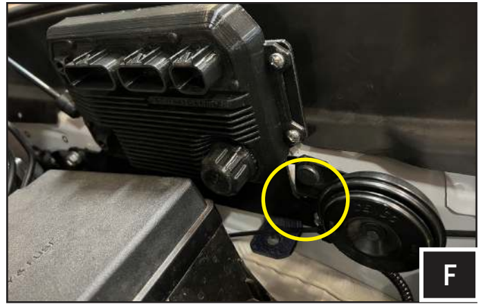
F. Position the horn and the ALPHA12 brackets and fasten using the horn bracket bolt. Do not tighten the bolt yet.
