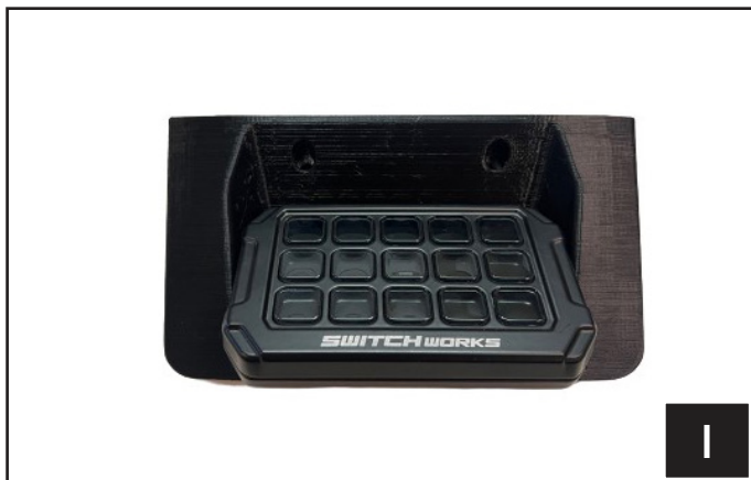
I. Picture above shows the orientation of the ALPHA12 controller to the fascia. Completed installation of the Gen 3 Toyota Tundra SWE12 15-Button Controller.
