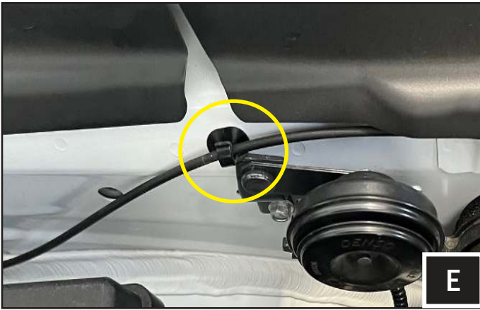
E. Remove the hood release cable from the cable clamp.
