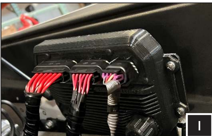
I. Connect the accessories to be used to the High and Low current harnesses and plug the harnesses to the brain module.
