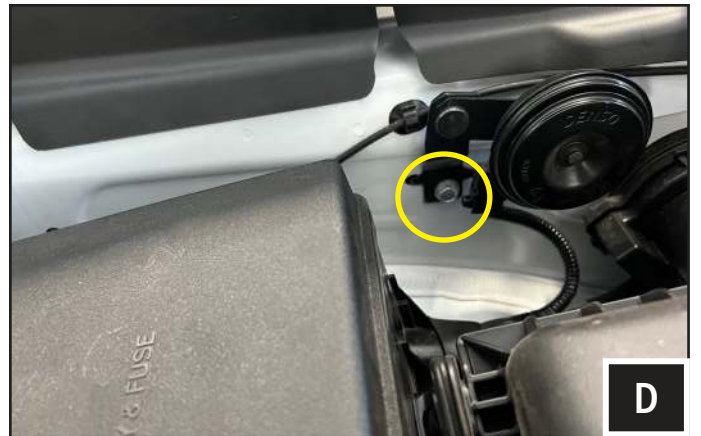
D. Remove the horn bracket bolt using a 10mm wrench.
