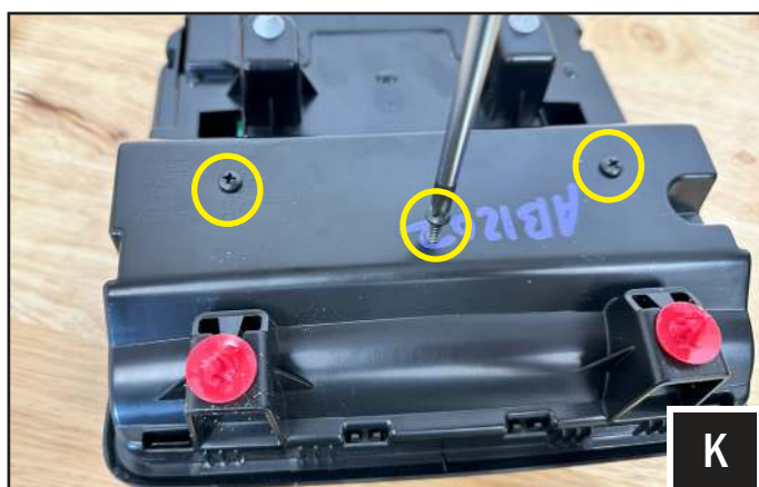
K. Flip the overhead console upside down and use (3) #7-19x3/4" Phillips screws (B-S1656) to secure the bracket.
