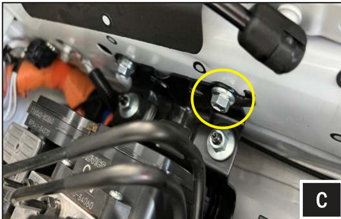
C. Remove the front bolt of the ABS pump bracket using a 12mm wrench.
