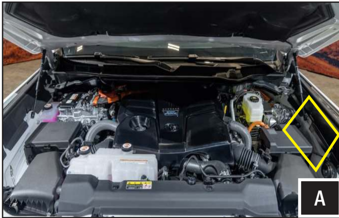
A. The SWITCH Works brain module is mounted on the driver side fender above the fusebox.
