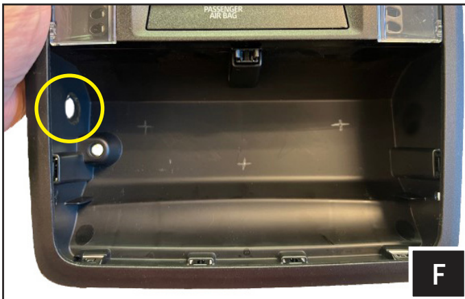
F. Drill a 16mm hole for the controller cable connector. Set aside the console for now.
