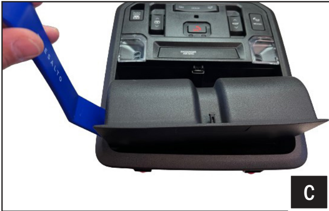
C. Remove the sunglasses holder. Open the sunglasses holder and use a pry tool to unsnap the left side (refer to picture above).
