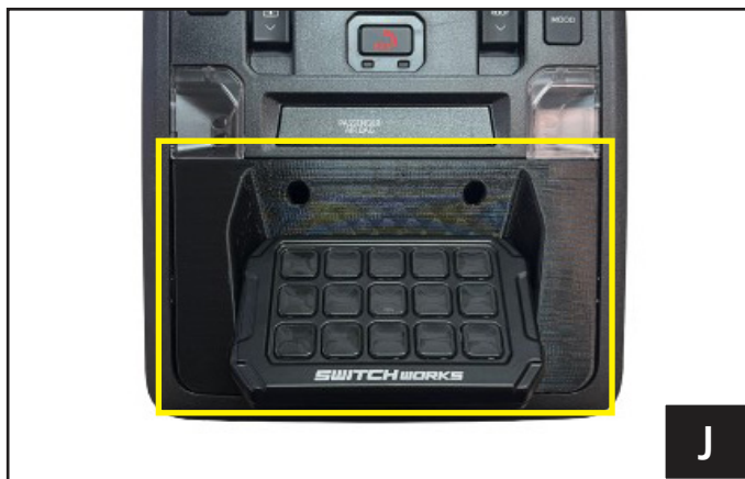
J. Insert the cable through the hole drilled on the overhead console and place the controller and bracket in the sunglass holder cavity.
