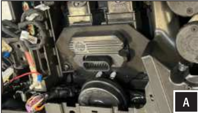
A. Find a suitable mounting location for the TANGO2 brain module. Secure the module with screws or zip tie it to a harness.
