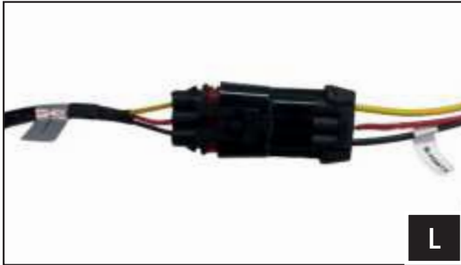
L. Plug the 3-pin connector of the Power Input Harness (B-H3413) to the X3 Turn Signal Main harness (B-H3271).
