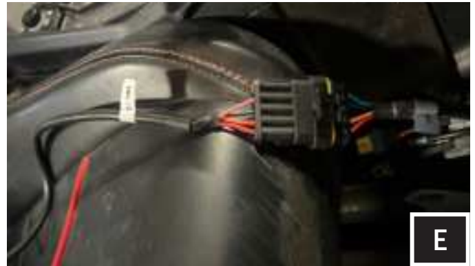
E. Run the TANG02 rear turn signal harness (B-H3205) to the rear of the vehicle. Use zip ties to secure the cable away from any moving parts or exhaust pipes.
