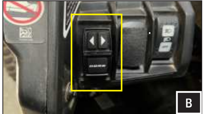
B. Use a vacant rocker switch mounting slot and insert the TANGO2 turn signal rocker switch. Run the cable towards the TANGO2 brain module.
