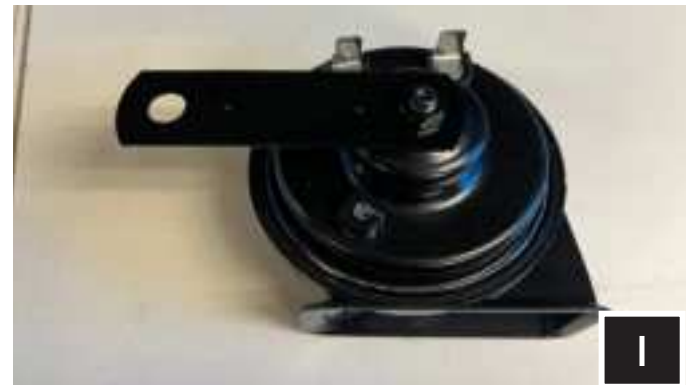
I. Mount the supplied bracket to the horn. Run the horn cable towards the desired horn mounting location.
