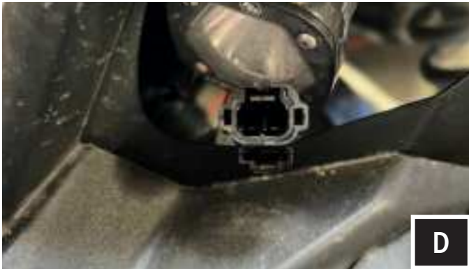
D. Route the front left and right turn signal extension cables to the front of the vehicle. Make sure to route the correct cable connector end that will plug to the LED lamp. Run the Horn power wires to the desired horn location.
