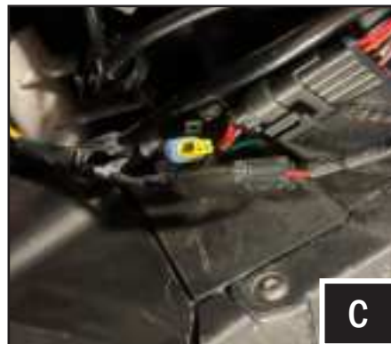
C. Plug in the controller cable, front turn signal extension cables (B-H2959) and rear turn signal harness (B-H3205) to the TANGO2 main harness (B-H3271).
