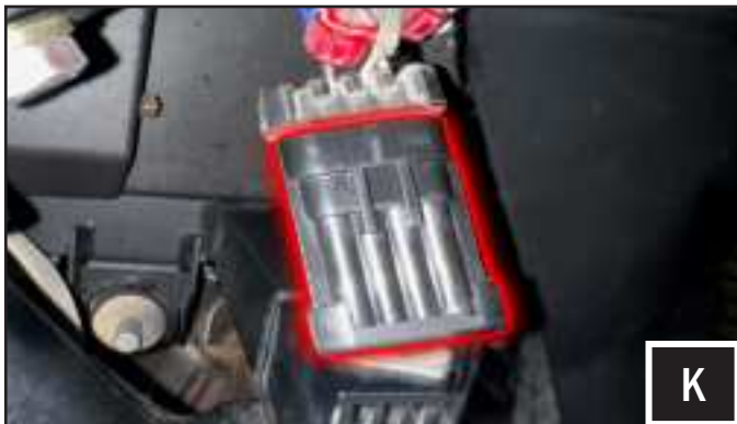
K. Plug in the provided dummy plug to the factory tail light connector to protect it from the elements.
