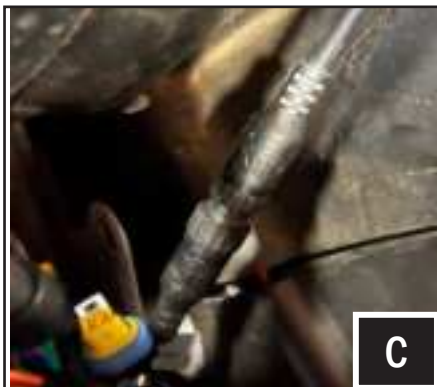
C. Plug in the controller cable, front turn signal extension cables (B-H2959) and rear turn signal harness (B-H3205) to the TANGO2 main harness (B-H3271).
