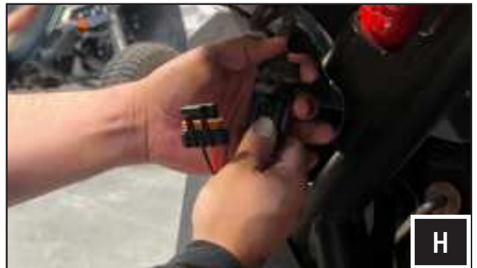
H. Unplug the factory tail light connector and plug it to the "PASS INPUT" connector of the X3 Rear Turn Signal Harness (B-H3205) that was ran to the back of the vehicle on step E.
