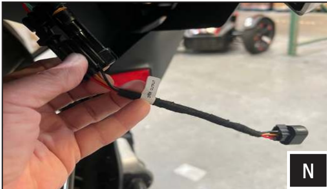
N. Plug in the KRX TS Adapter (B-H3122) to the B-H3112 “DRIVER OUTPUT” connector and plug the other end to the tail light. Use zip ties to secure the harnesses.
