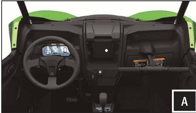
A. Locate a suitable mounting location for the TANGO2 Turn Signal module. Secure the module to a panel using screws or zip tie it to a harness.
