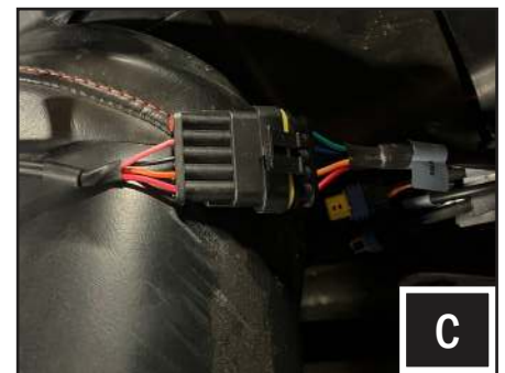
C. Plug in the controller cable, front turn signal extension cables (B-H2959) and rear turn signal harness (B-H3112) to the TANGO2 main harness (B-H3271).
