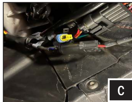
C. Plug in the controller cable, front turn signal extension cables (B-H2959) and rear turn signal harness (B-H3112) to the TANGO2 main harness (B-H3271).
