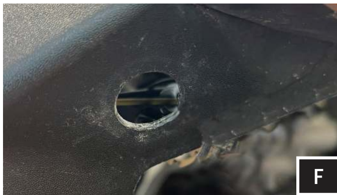
F. Drill a 3/4" hole in the front of the vehicle for the front turn signal LED lamp. Refer to the viewing angle diagram on page 7 for proper turn signal LED lamp placement.
