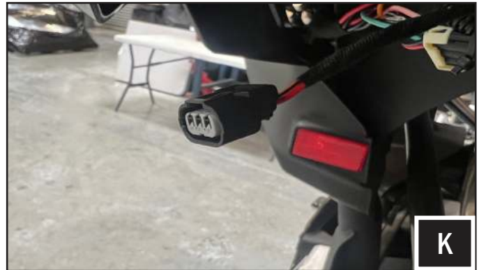
K. Run the KRX Rear Turn Signal Harness (B-H3112) to the rear of the vehicle. Begin installation on the passenger side tail light. Unplug the passenger tail light connector. See wiring image below for the passenger side connections.
