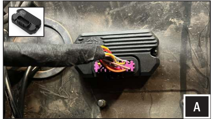
A. Locate a suitable mounting location for the TANGO2 Turn Signal module. Secure the module to a panel using screws or zip tie it to a harness.
