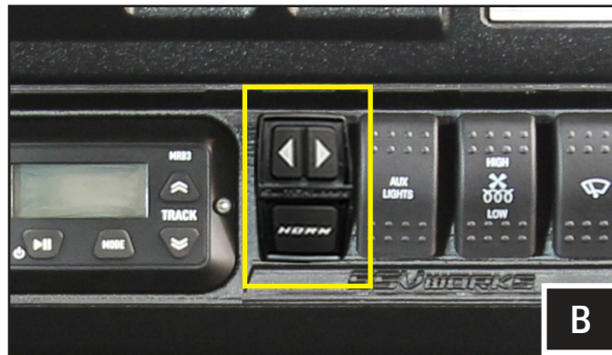
B. Use a vacant rocker switch mounting slot and insert the TANGO2 turn signal rocker switch. Run the cable towards the TANGO2 brain module.
