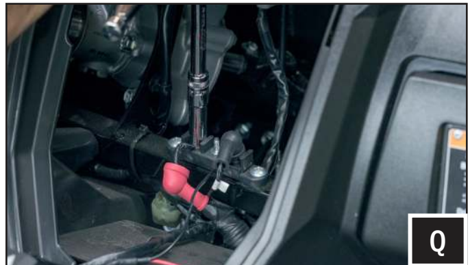
Q. Run the BATT, ACC and GND wires of the Power Input Harness (B-H3413) to the factory busbar and screw in the ring terminals to the corresponding battery, Accessory and Ground studs.
