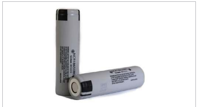
Figure 11: 18650 Cells from Ring Battery Pack
