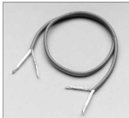
SC-182: Low inductance (42 nH/ft) coaxial cable for minimizing test lead impedance in circuits using fast transient response power supplies. The cable is sold by the foot and comes without connectors.
