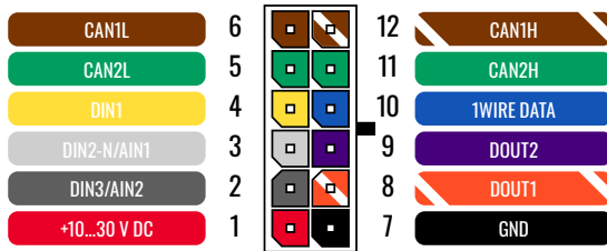
FMB150-QJIB0 pinout
