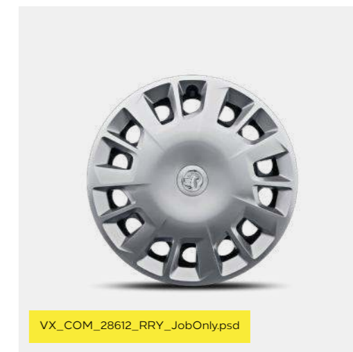
16" steel wheel with full-diameter wheel trim
