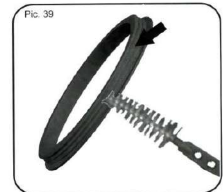
clean the bowl gasket along all the edges as shown in Picture 39.
