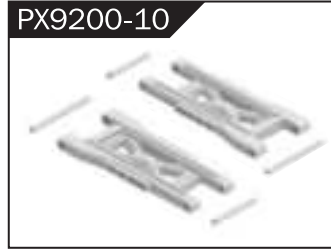
Lower Suspension Arm
