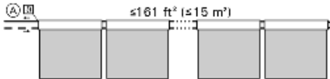
(A) Collector temperature sensor
