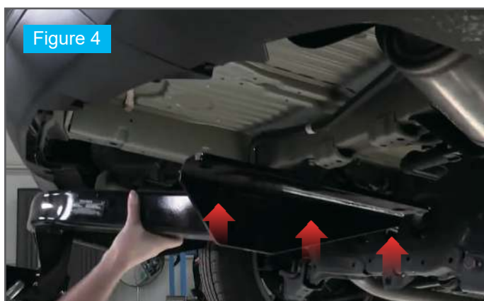
Lift the trailer hitch by tool or ask your partner to assist you.
