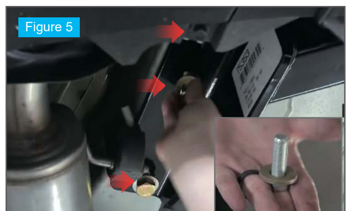
Take out hex bolts and spring washers slightly tighten the hex bolts.
